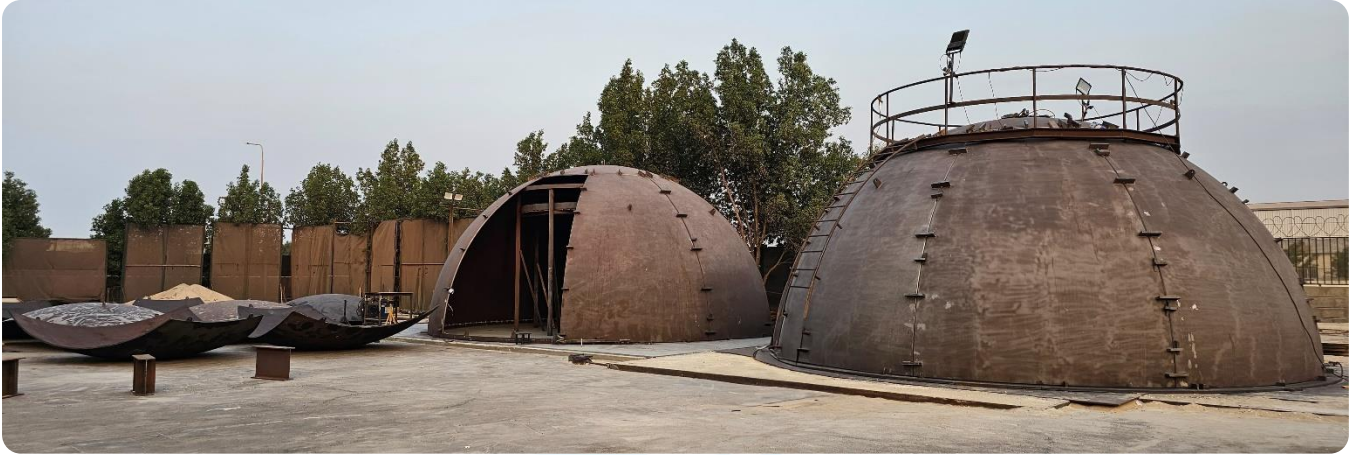
Dish Head Forming – 9000mm dia 35 mm thick
