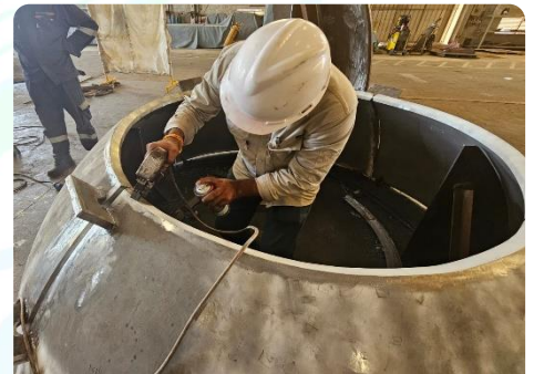
Crown and Petal – HemiSpherical Dish Head MPI Test on the surface and bevel edges
