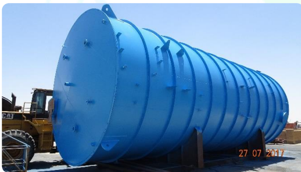
200m3 Water Storage tank
