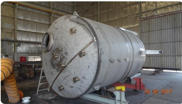
Phase Separation Tank
