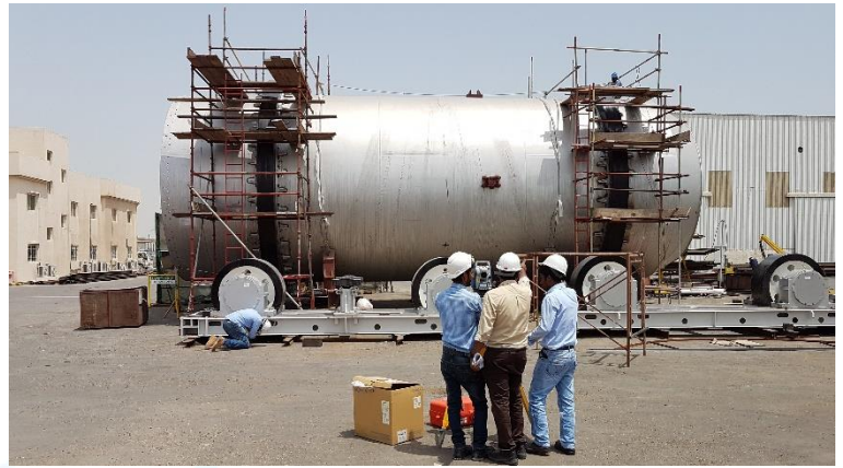
Fabrication & Welding Kiln
