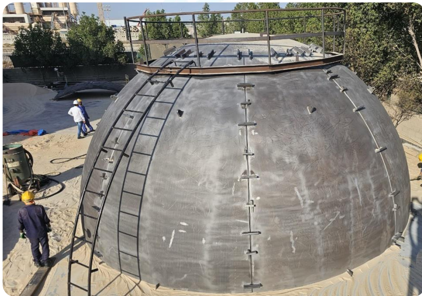
Dish Head Forming – 9000mm dia 35 mm thick
