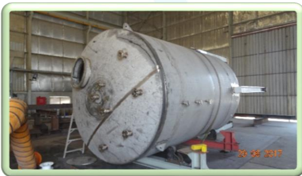
Phase Separation Tank
