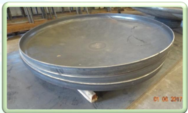
FGE & AW tank dish fabrication
