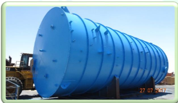
200m 3 Water Storage tank
