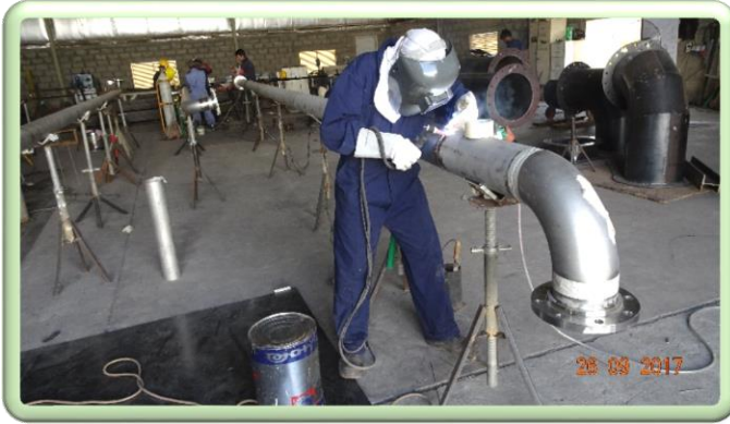
CS & SS Pipe fabrication completed
