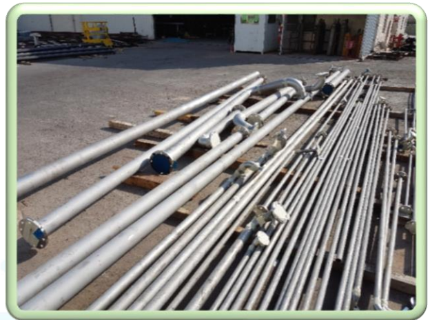
CS & SS Pipe fabrication completed
